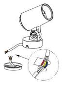
5. Connect the power cord with the power cord of the lamp, and then tie it with waterproof tape (waterproof measures mube taken)
