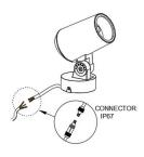
7. Put the power cable and the power cord of the lamp into the IP67 waterproof joint
