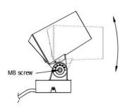
7. Loosen the M8 cup head screw of the base, adjust the Y axis Angle of the lamp and then lock the screw
