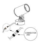
8. Connect the power cable, and then lock the waterproof connector
