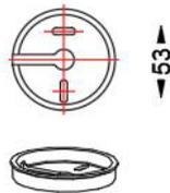
2. Drill two holes on the wall or floor according to the hole position of the base bracket, and put rubber plugs or wood block into the hole
