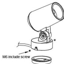
1. Loosen M6 screw and remove lamp base bracket
