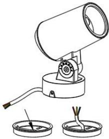
4. Drill a threading hole in the center of the base bracket and the wall, and then put the power cord of the lamp into the center of the base bracket or connect a power cord out of the wall
