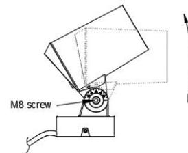
6. Loosen the base M8 cup head screw, adjust the Y axis Angle and then lock the screw
