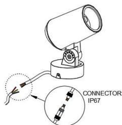
7. Put the power cable and the power cord of the lamp into the IP67 waterproof joint
