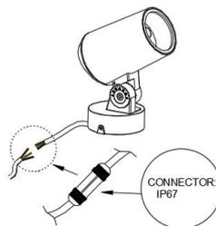
8. Connect the power cable, and then lock the waterproof connector
