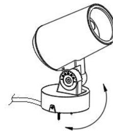
6. Put the long power cord into the base, and then put the lamp into the base bracket, and adjust the X axis Angle of the lamp and then lock the screw.
