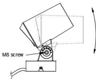
7. Loosen the M8 cup head screw of the base, adjust the Y axis Angle of the lamp and then lock the screw
