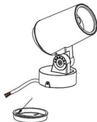
4. Insert the power cable into the side hole of the base bracket
